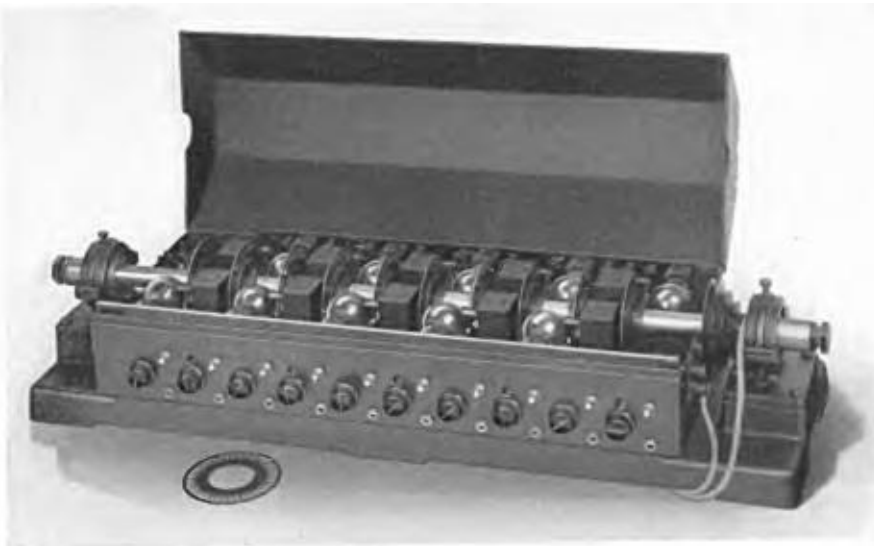
FIG. 23. Ten disk optical tone generator.
